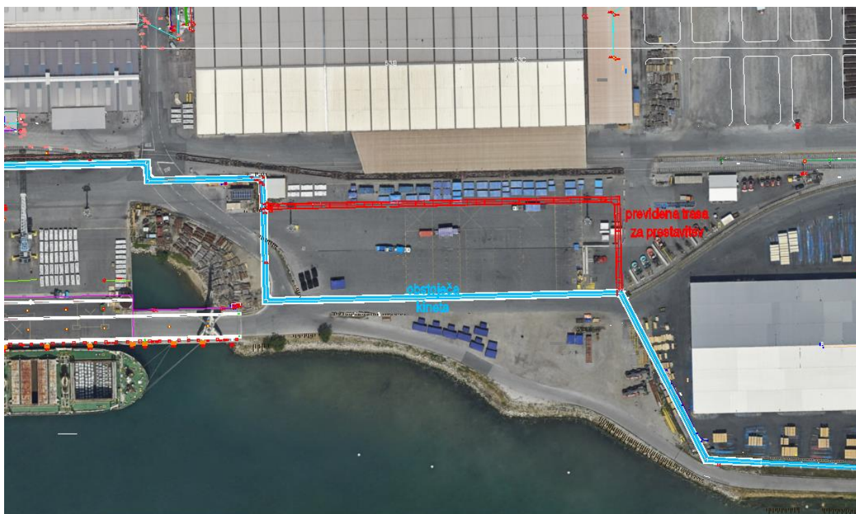
Figure 10: Pier II - ortho photo of the existing (blue) / planned (red) route of the pipeline trench
